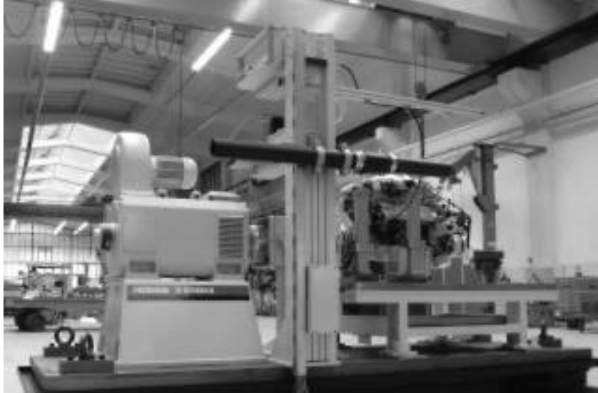
Figure A-2. Titan Engine Dyno test stand installation by Horiba Automotive Test Systems
