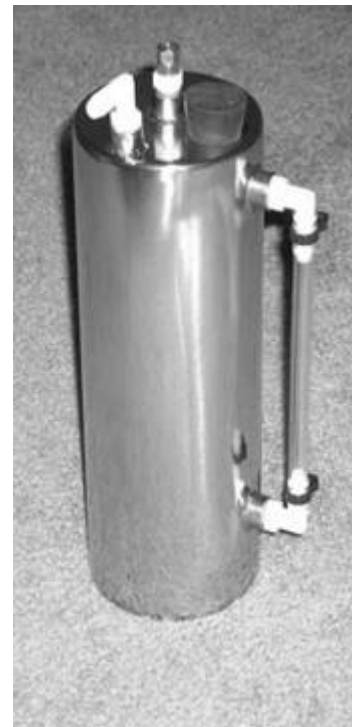
Figure 4.2. SS-40 HHO generator
